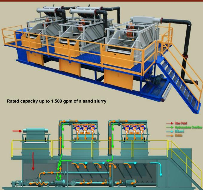
Power Requirements 3 Phase 480 V, 60 Hz 250 Full Load amps
