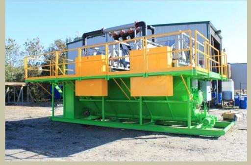
The TCS-750 system rated capacity up to 750 gpm of a sand slurry
