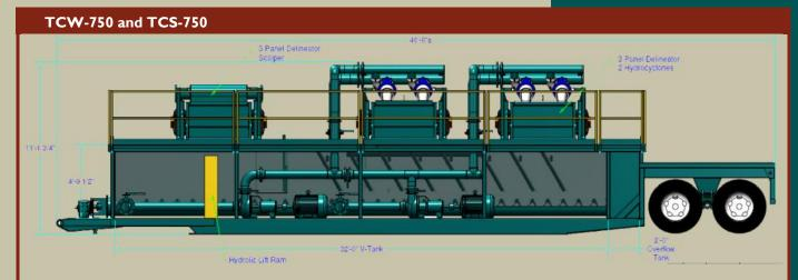
Power Requirements 3 Phase 480 V, 60 Hz 125 Full Load amps **Operating Dimensions:** 46'-6" L X 8'-6" W X 11'-2" H **Transportation:** (1) Legal Load with 3 Panel Shakers **Setup Time:** (1-2) Hours, No Crane Needed **Operators Needed:** (1) Equipped with Hydraulic Lift Ram for easy loading and unloading
