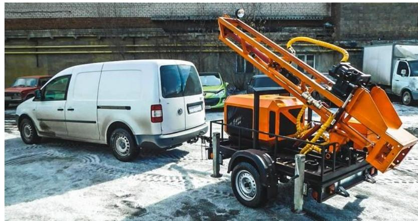
The design capacity of the mini-installation (loose and medium erosion) from 5 to 22 m<sup>3</sup>/hour for solid washing and enrichment.
