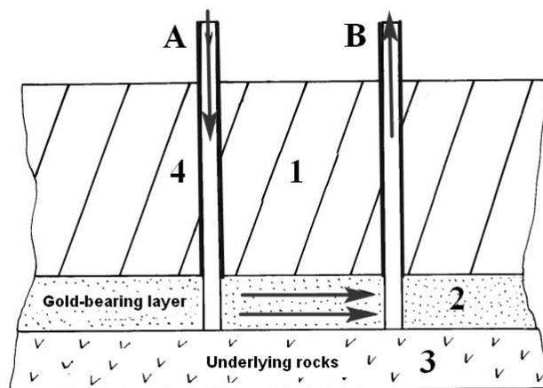
Initially, in the array 1, a bush of technological wells A and B is drilled, opening the formation 2 of compacted gold-bearing rocks to the underlying rocks 3. The wells are cased with pipes 4, equipped with heads, hydraulic fracturing between wells A and B of formation 2 and acidification are carried out. Then, efficient and environmentally friendly solutions of alkali and alkaline earth metal oxychloride are
