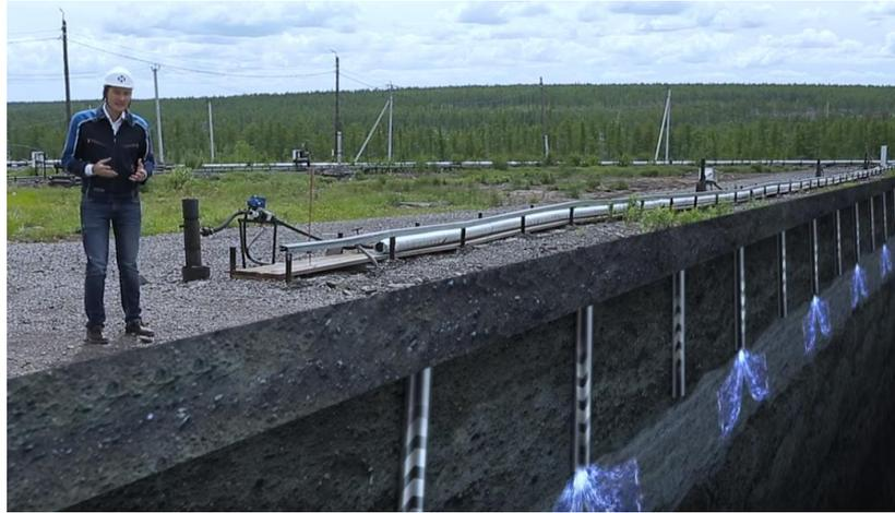
At the pilot block of Underground Leaching with a solution capacity of 15-25 m<sup>3</sup>/h, taking into account the hydrogeological conditions of the site, an infiltration-filtration system for borehole mining of the ore / formation massif with airlift elevation of productive solutions was developed and implemented. Coal sorption technology has been adopted to extract gold from solutions.
